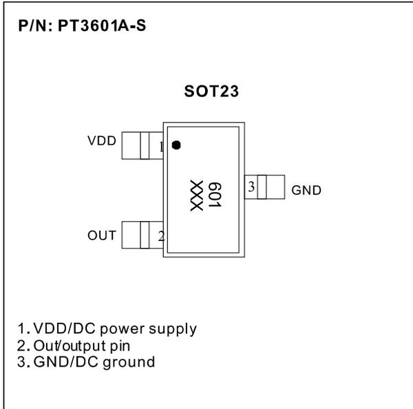
The PT3601A is designed for magnetic actuating using a bipolar magnetic field. The built-in dynamic offset cancellation of pre-amplifier stage achieves optimal symmetrical magnetic sensing. This Hall effect IC is optimal for DC brushless motor application. The supply voltage range is from 2.5V to 18V and maximum output current is 25mA.
